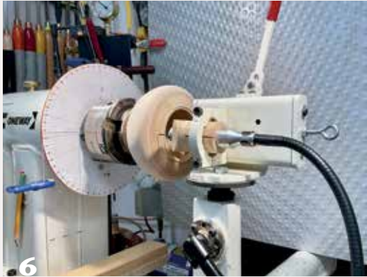
6 The author uses a Oneway Drill Wizard to drill the holes for the hand-stitching. The drill bit is at spindle height. Drill a new hole at each indexed interval (with the lathe off).
