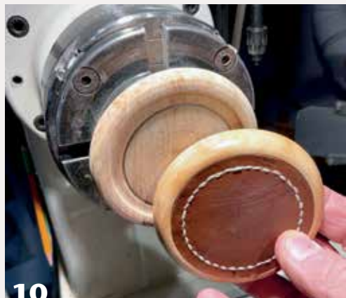
10 Mounted in the chuck is a new box lid. Turn a recess to accept the thickness of the leather round. The author holds a completed example.
