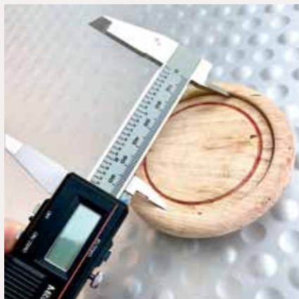
11 A caliper is used to measure the width of the recess, then the author uses a circle cutter to cut the leather to fit.
