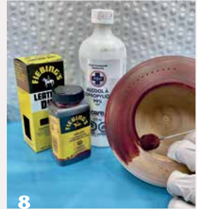
8 Leather dye works well to color the wood prior to stitching. A contrasting color to the thread gives a dramatic effect.
