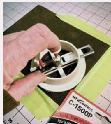
11 A caliper is used to measure the width of the recess, then the author uses a circle cutter to cut the leather to fit.
