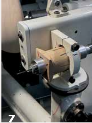
7 A Foredom tool serves as a drill. It is clamped to the Drill Wizard using a shopmade wood collet.
