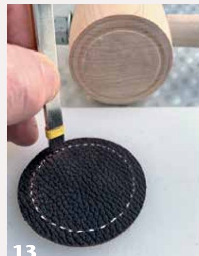
13 A pricking iron is used to indicate hole locations for hand-stitching leather thread into the round of leather.
